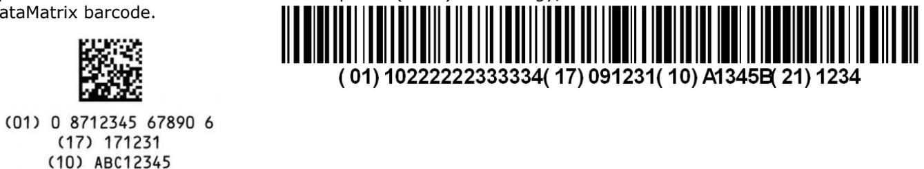
Figure 2.2 GS1 DataMatrix and GS1-128
